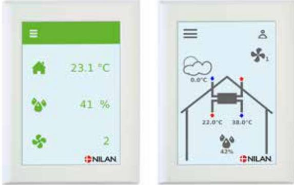
The Comfort 300LR is controlled using its CTS 602 HMI touch panel, featuring a wide range of functions, e.g., menu-controlled operation, weekly programme settings, filter monitor with timer, fan speed adjustment, summer bypass, supply-heating element control, error messages etc.
