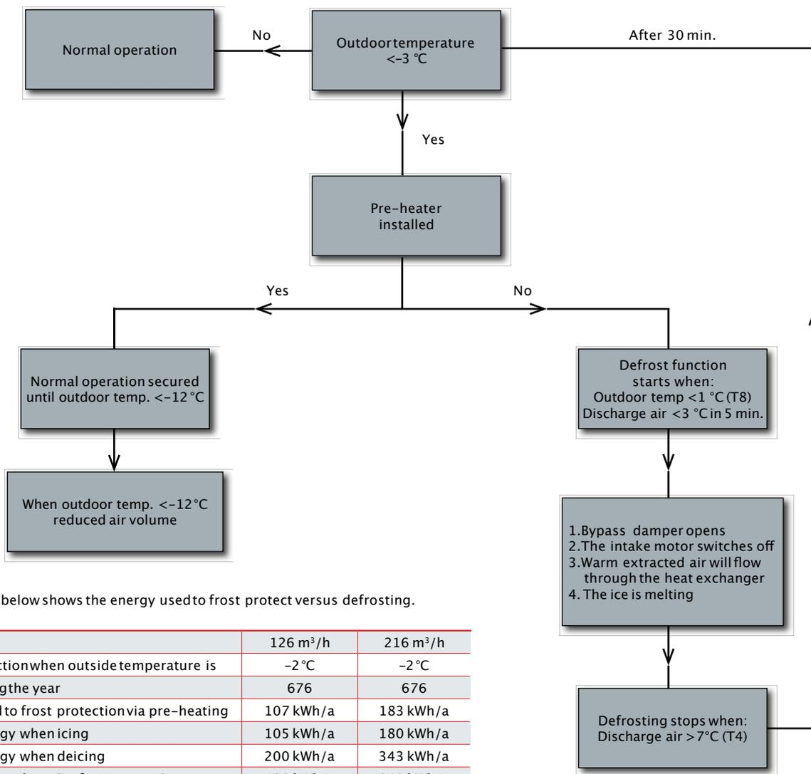
The example below shows the energy used to frost protect versus defrosting.
