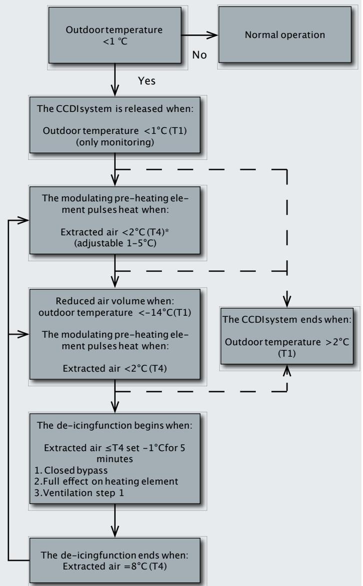
NB! All temperature settings are adjustable. On adjustment, they must be matched to the conditions in the home and the local climate.
