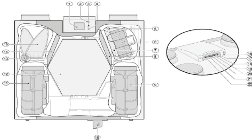
The device shown above is a left-hand version; in the right-hand version, the connection of the pre-heater, bypass valve and the siphon are mirror-mounted.
