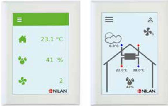
The VPL28 is controlled using its CTS 602 HMI touch panel, featuring a wide range of functions, e.g., menu-controlled operation, weekly programme settings, filter monitor with timer, fan speed adjustment, summer bypass (free cooling), supply-heatingelement control, error messages etc.
