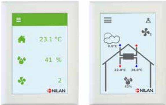
The Comfort 5000 is controlled using its CTS 602i HMI touch panel, featuring a wide range of functions, e.g., menu-controlled operation, weekly programme settings, filter monitor with timer, fan speed adjustment, summer bypass, post-heating element control, error messages etc.
